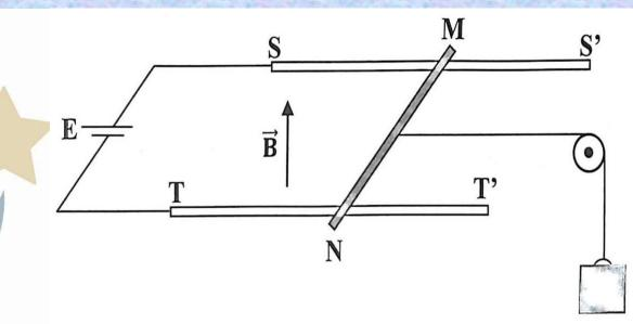
On these two rails, a metal rod MN can slide without while remaining  $\bot$  to the rails.
